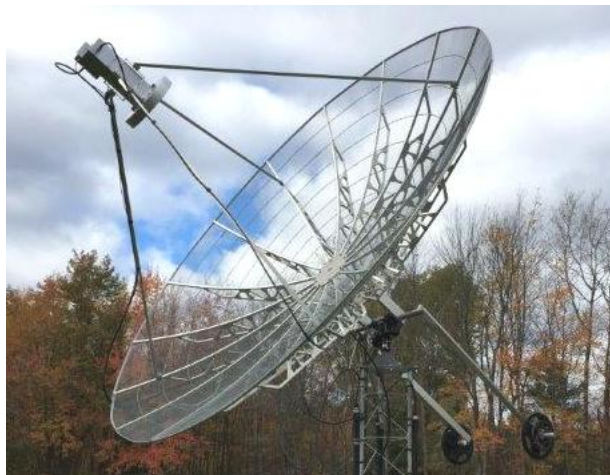
NC11 's 4.5 m dish used to score 65x37 from NA on 1296 in Nov
