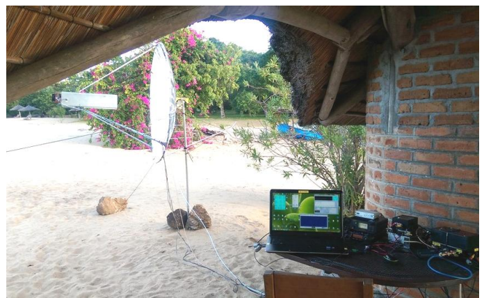
7Q7EME's 1.5 m dish with 1296 feed as seen from their operating position
