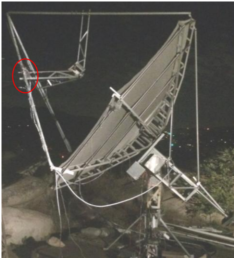
WA6PY new 6 cm feed with TWT on support pole
