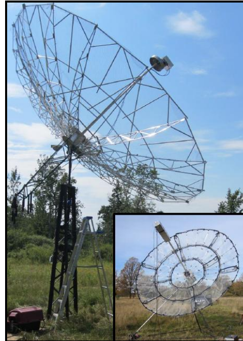
KNOWS 6 m used 70 cm & new 3.2 m stress dish for 23 cm
