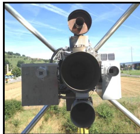
HB9Q's feeds (23, 13,9, 6 & 3 cm offset mounted on his 10 m
