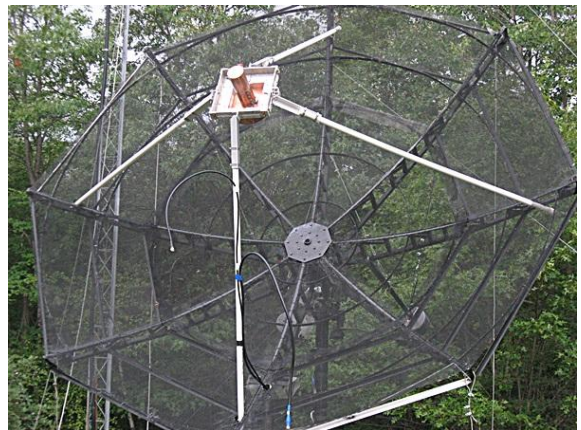
WA2FGK's 3 m dish and feed for 13 cm
