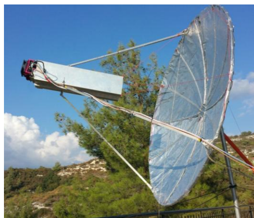
5B/DL2NUD 1.5 m dish with 23 cm feed in place
