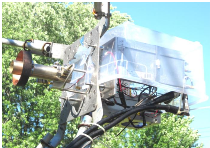
WA9FWD's feed and SSPA box
