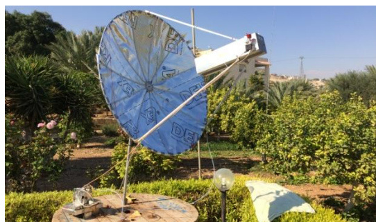
E44QX/E44HP 1.5 m dish with 23 cm feed
