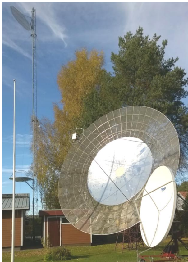
OH2DG dishes: periscope dish for 1.2 to 23 cm, 8 m dish (4 m solid center) for 3 to 70 cm and 3 m dish for 1.2 cm.
