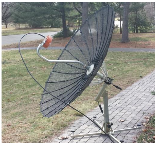
W2HRO's 1.8 m Toki umbrella dish with linear feed used to work HB9Q on 1296
