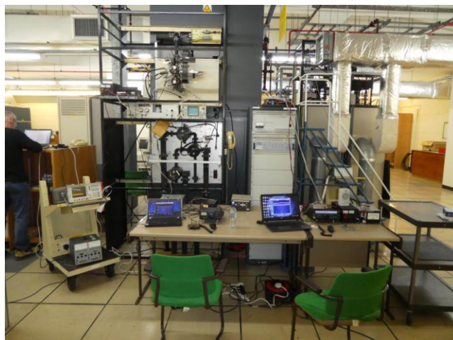
GB6GHY shack with the 9 cm system on the left and the 6 cm system on the right. Transverters are located above head level close to the waveguide feeds.
