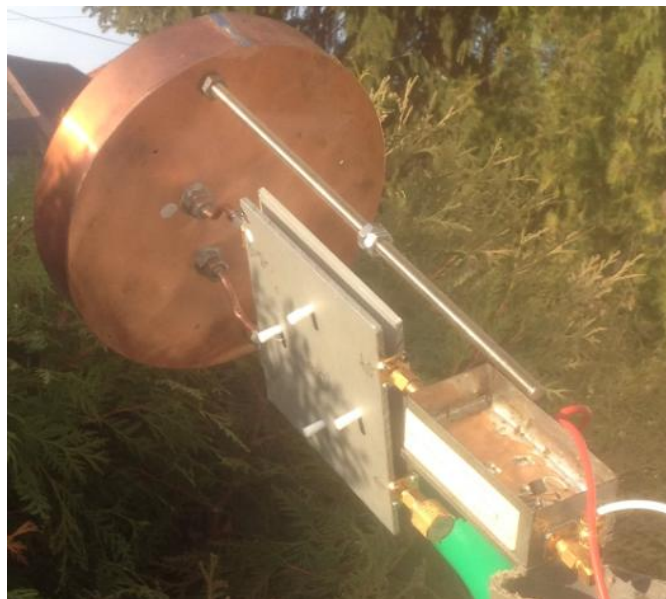
G3WDG coupler attached to patch feed
