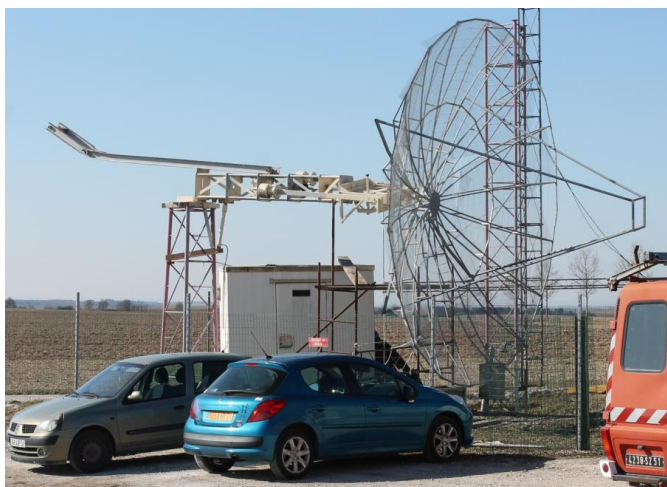
Dish at F6KHO to be used on 23 cm EME
