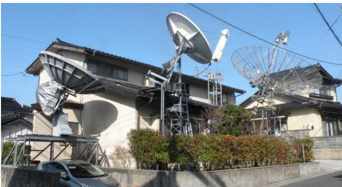
JA4BLC's 3 dish in simultaneous operation: (R to L) 6 m dish on 1296 and 2400, 2.4 m offset dish on 10 GHz and 3 m Cassegrain dish on 24 GHz.
