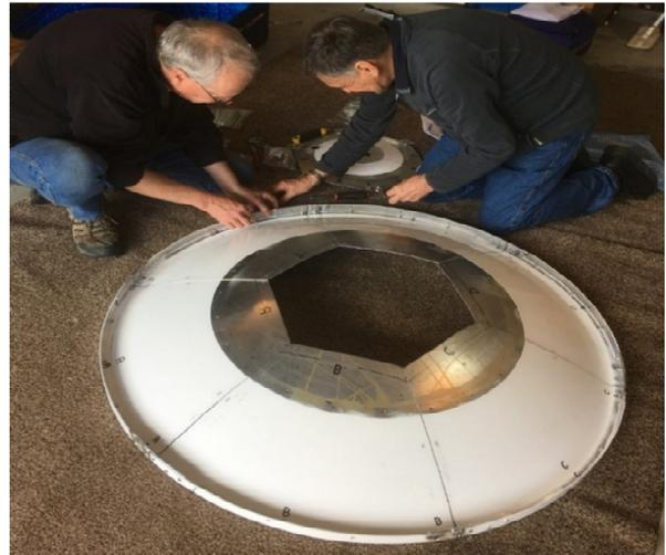
Roger ZL3RC (left) and Rex VK7MO (right) assembling the 1.13 m flyable dish. This was cut-up from a solid aluminum dish with a jigsaw - [See also Oct NL page 7].
