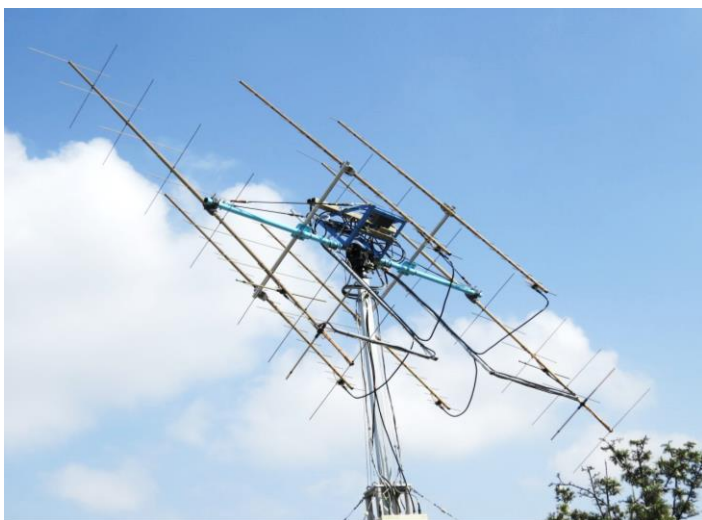
4Z5CP's 70 cm 4 x 16 el I0JXX yagi array
