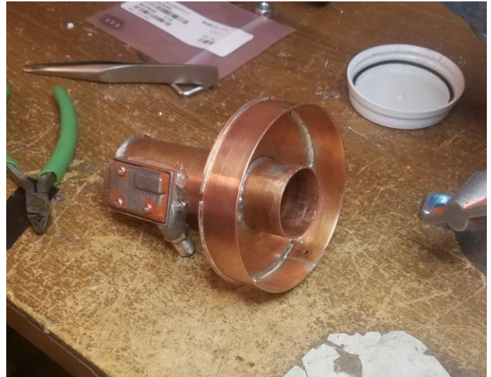
K5DN experimental 3 cm horn, LNA/down converter
