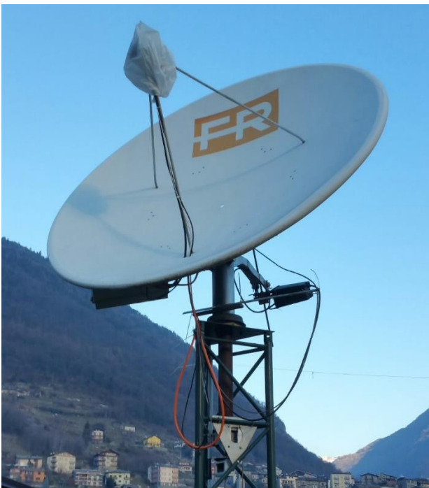
IW2FZR's 1.8 m dish used on 3 cm with 20 W TWT
