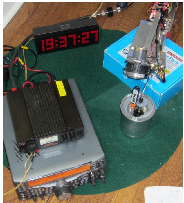
KN0WS calorimetric power testing on 3 cm
