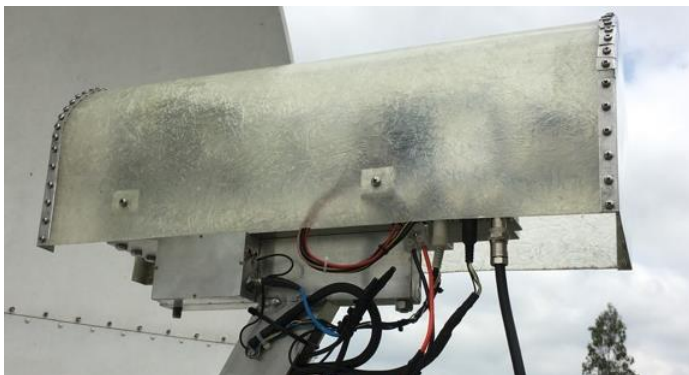
PY2BS 10 GHz feed arrangement
