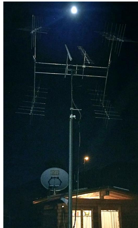
IW2FZR's EME antennas at home QTH with 1.8 m dish
