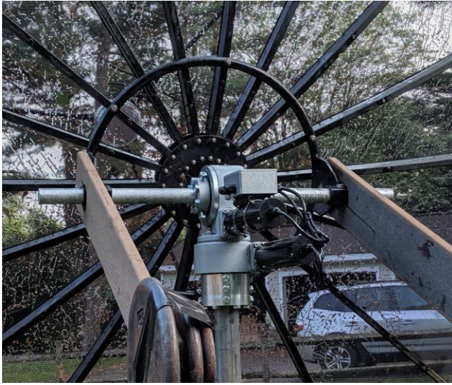
W2HRO's Sunslew slew drive rotor for his 4 m dish
