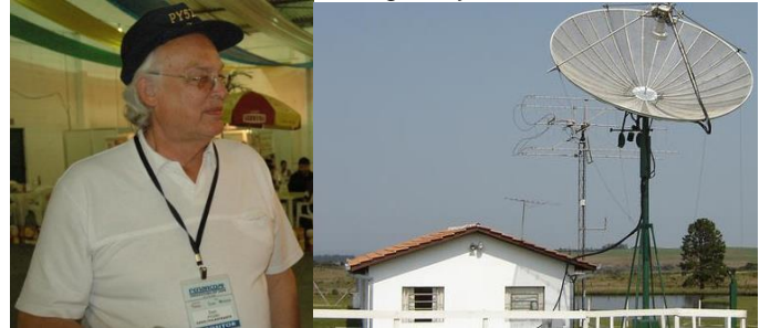
PY5ZBU and EME QTH with 5 m dish used on 1296 and behind 432 yagi array
