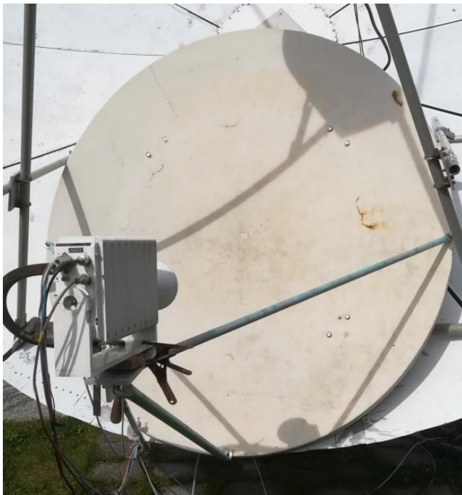
DL4DTU 1.8 m offset dish with 3 cm feed.
