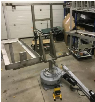
Sunslew Slew Drive ZE12A-78-RC-24H50200 & Linear Actuator SS-15000-800-2.8-24 used to point dish
