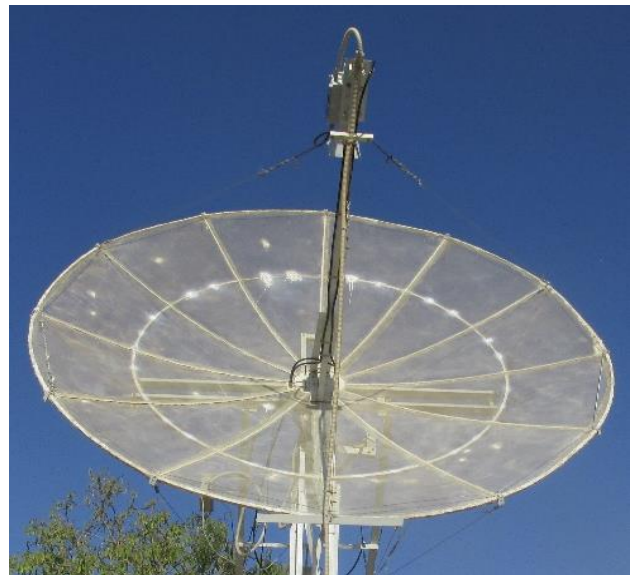
4X4AJ's 3 m HB dish with 9 cm feed in place
