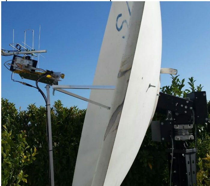
CT1BYM dish with 24 GHz feed in place
