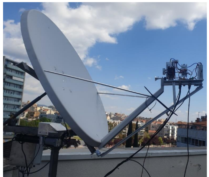
EA3HMJ's 47 GHz experimental EME station
