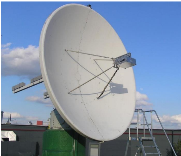
3.7 m dish used by DB6NT for EME on 24 GHz
