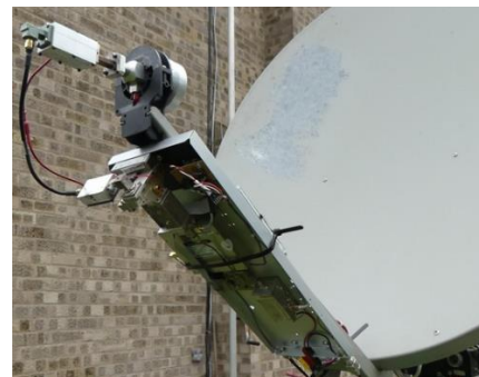
G4BAO's dish used for EME experiments on 24 GHz
