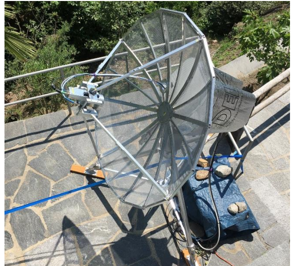
HB9CRQ grid dxpedition 6 cm feed in 1.8 m dish
