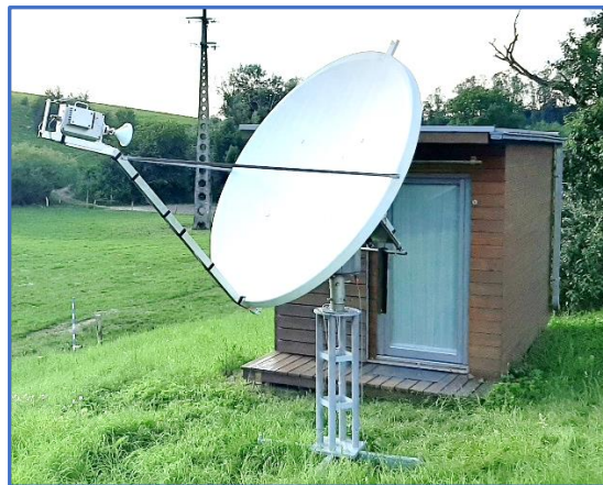
OK2AQ EME QTH with a 1.8 m offset dish that replaced a 1.2 m dish used until this spring
