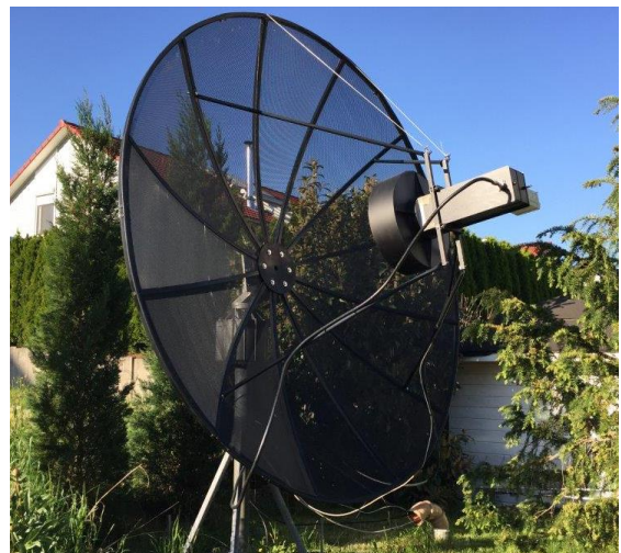
DJ3JJ's 2.5 m dish (f/d 0.36) with RA3AQ 23 cm feed
