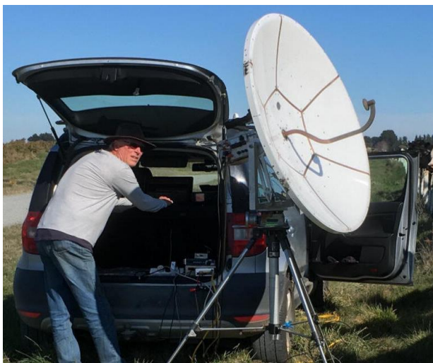
ZL3RC's 3 cm rig that was used for the far end of long distance QSO with OK2AQ
