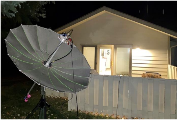
KB7Q's stealth, folding 1.6 m dish and path feed
