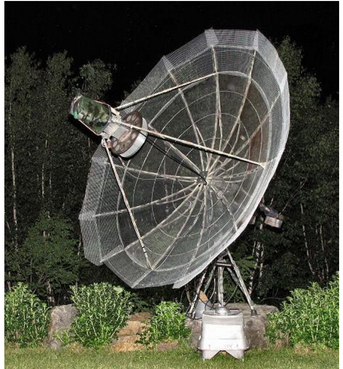
KA1GT's 3.15 m dish (expanded from 2.4 m) with around 240 W at the feed used in the EME contest
