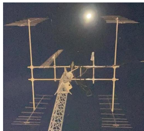
HI8DL is QRV on 432 with a single 9 WL M 2 yagi in the middle of 4 x 2 m yagis and 75 W from the Dominican Republic – (see OK1KIR's report)
