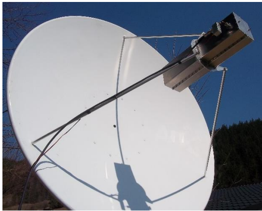
OK2PE's new HB 3.2 m dish used on 23 cm
