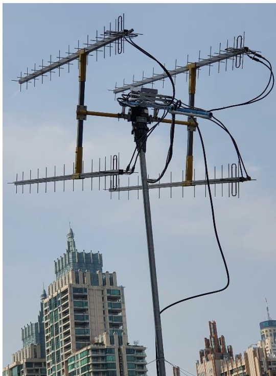
HS0ZOP's 4x15 el LFA-JT yagis & ~ 500 W at feed
