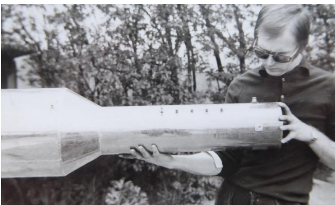
W2IMU circular pol dual mode horn feed used by Jan
