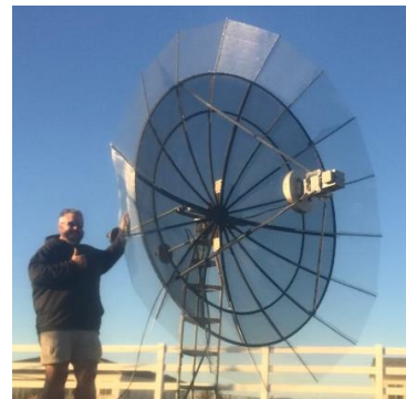
N1AV with 3 m dish extended to 4.2 m
