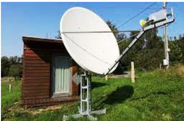
OK2AQ's 1.8 m offset dish and 50 W SSPA – 26 QSOs on 3 cm in the MW part of the ARRL EME Contest
