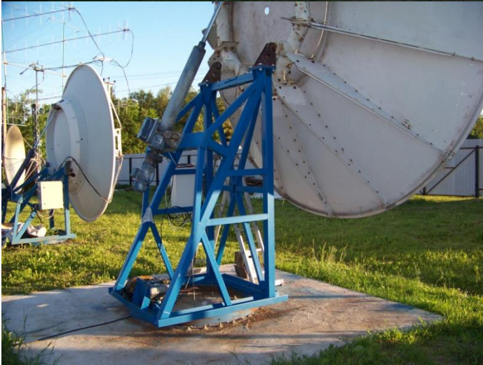
Dishes used by UA5Y during the MW contest. The 5 m dish at top was used on 13 cm
