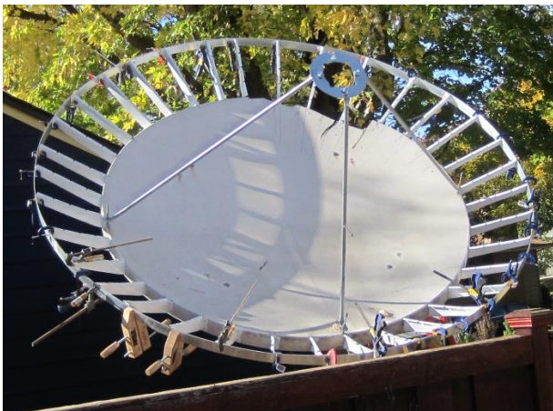
KNOWS has extended his 1.8 m home dish to 2.4 m and maybe QRV with it on 1296 in Nov
