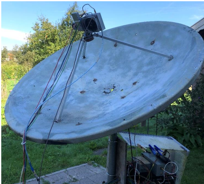
G3WDG prime focus 1.2 m dish with feed mounted WG switch, PA and LNA
