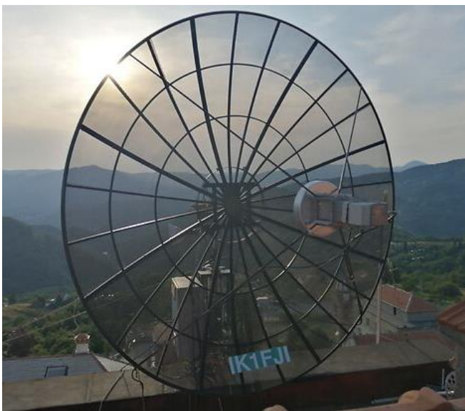
IK1FJI's new 3.8 m dish with 1296 feed
