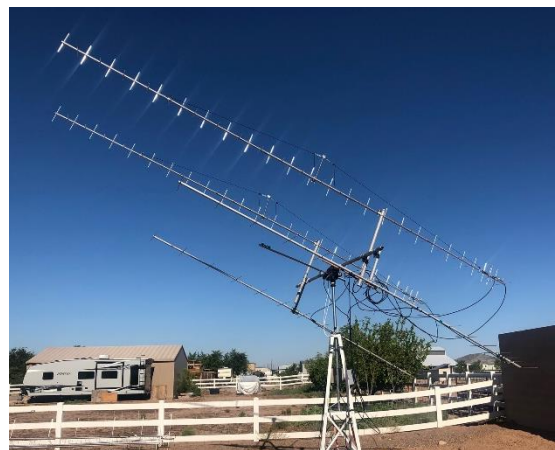
N1AV's 432 2 x H & V 25 el yagi array & 222 yagi
