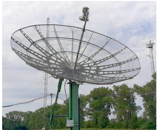
OK1UGA's 6 m dish on 23 cm with upgraded feed
