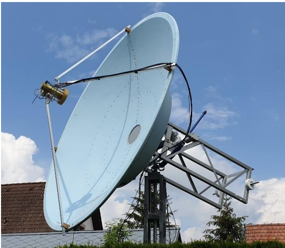
OM6AA's new 3.6 m RFS dish on 13 cm
