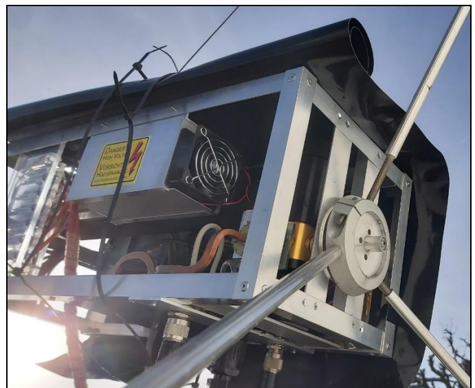
DL7YC's resized 47 GHz TWT (42 W) Hughes 8901HA at feed of his 2.4 m dish – note the size of the actual feed.
