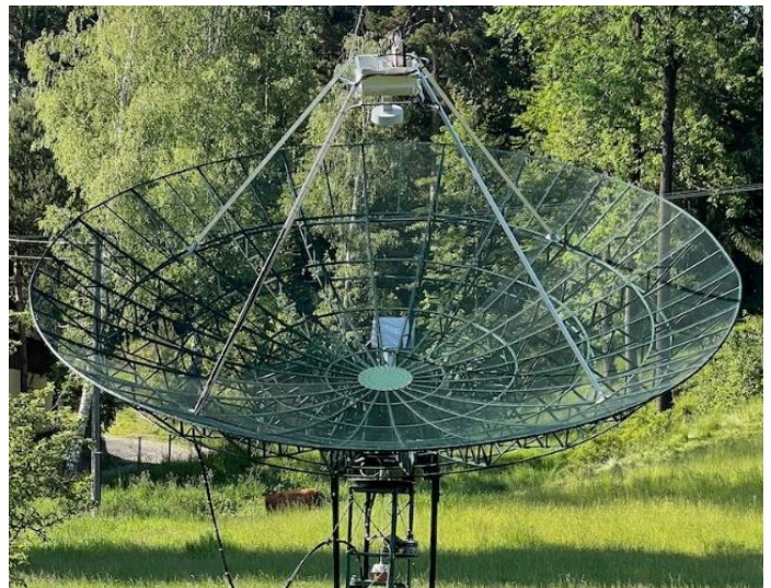
SP9VFD is now on 13 cm with his 6.4 m HB dish
