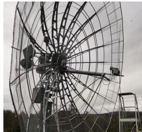
DL6SH's 8 m mesh dish with 6 cm feed
