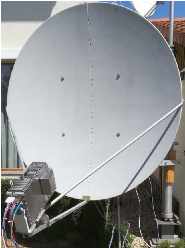
1.8 m dish used for 9, 6 and 3 cm at OJ0EME
