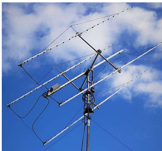
PA5Y 432 4 x PA432-23-6B yagi array used to win ARRL Contest single Op all modes all bands
