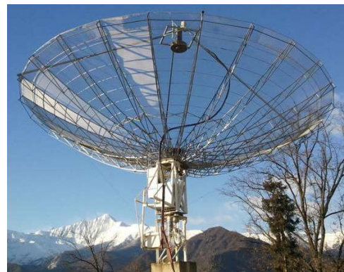
IZ1BPN 8 m dish with 23 cm feed
