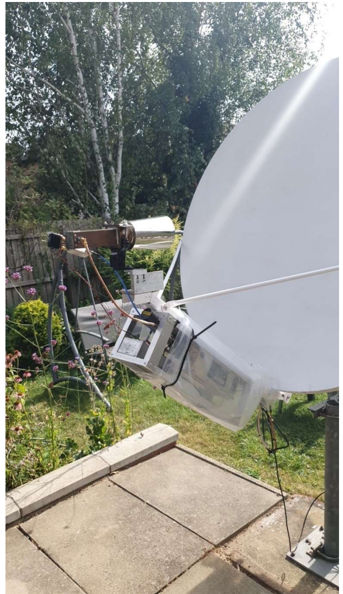
Figure 8- G4BAO 5.7 GHz feed system
