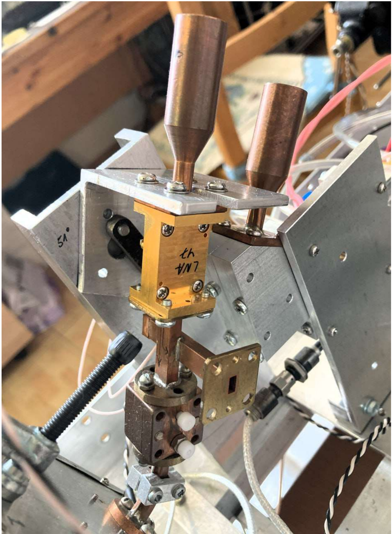
Figure 26 - RW3BP head unit rx
