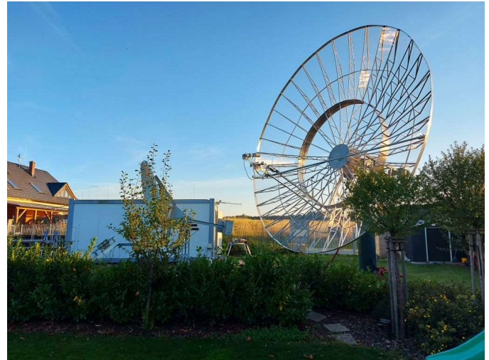
Figure 14 - OK1DFC 8m + 2.4m offset dishes for 13-3 cm
