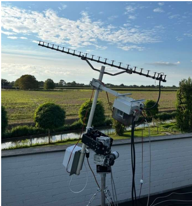
Figure 27 - PA3DZL 23el 1.75m 15.8 dBd setup
