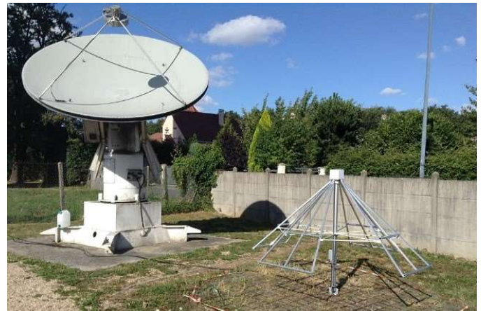
Figure 6 - F1EHN 3.3m dish + 21cm astronomy feed
