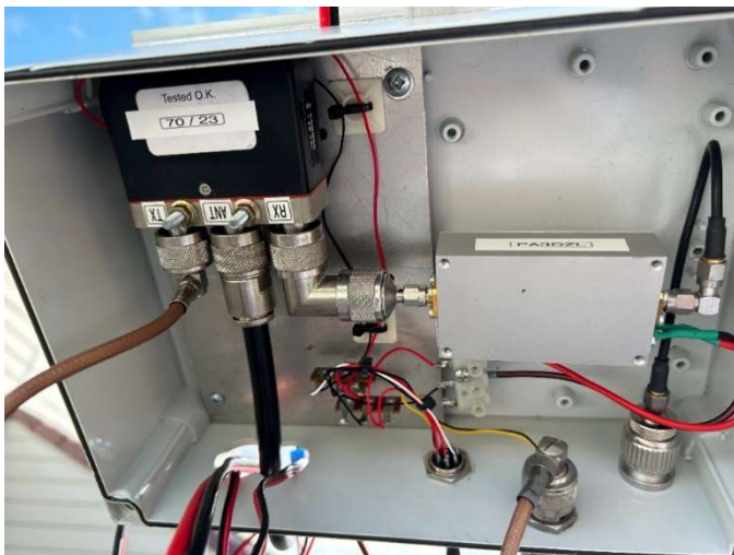
Figure 28 - PA3DZL N coax switch + preamp
