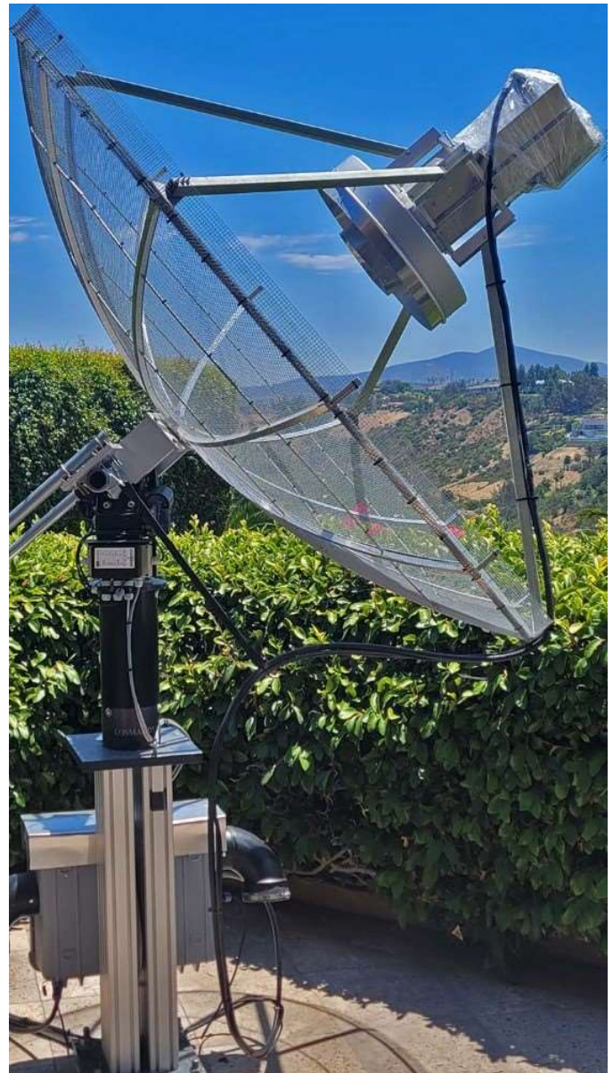
Figure 26 - KB2SA optimised 1.9m dish
