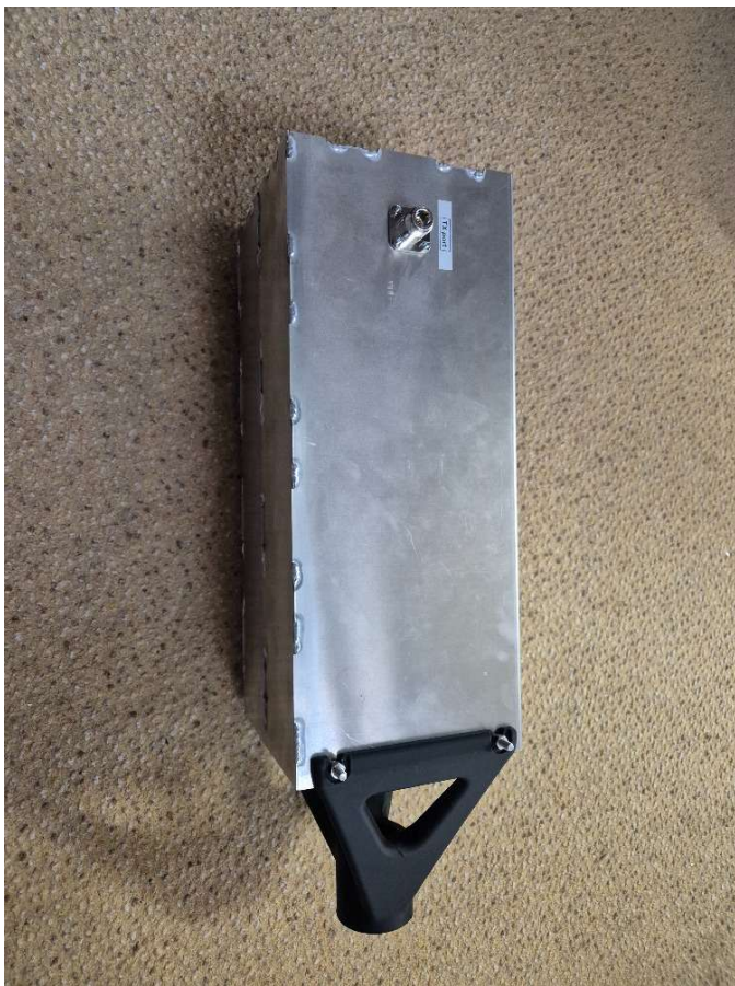
OK1DFC 23cm feed side view
