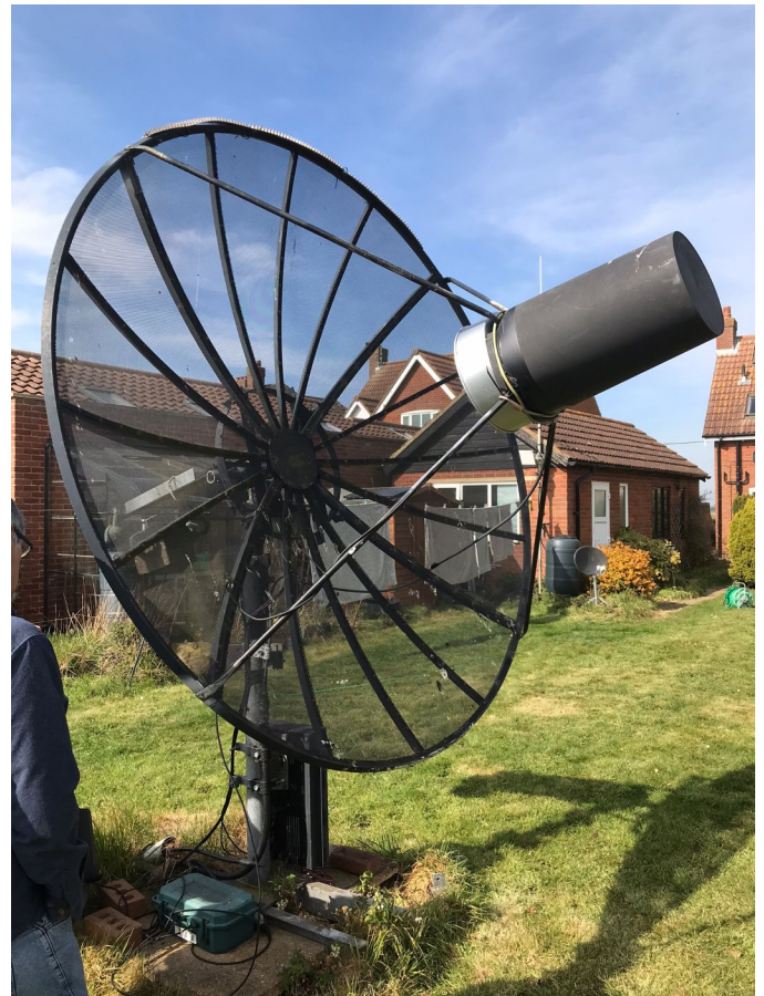
G4DDK 2.3 m dish with 23 cm feed
