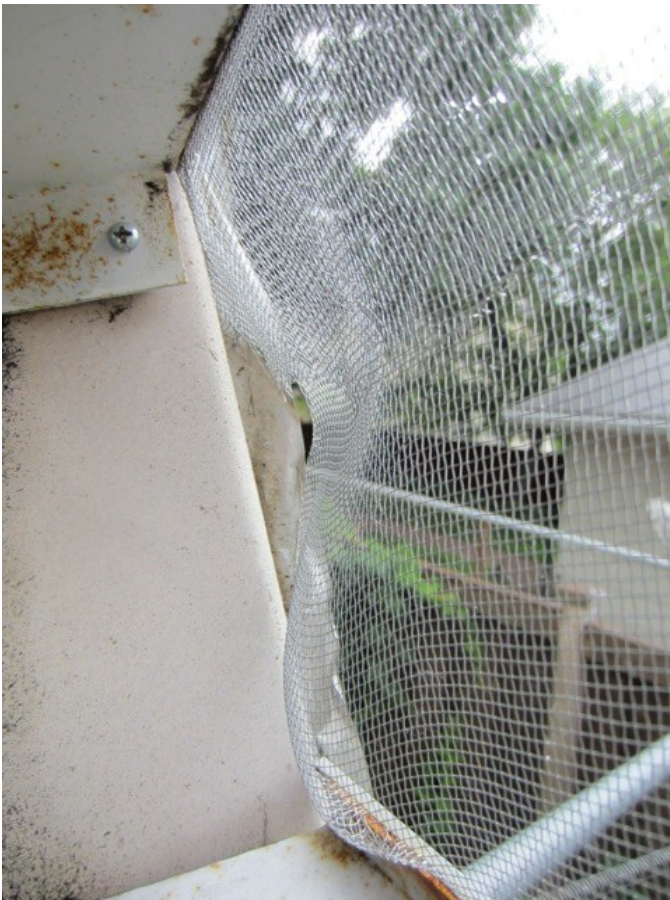
KNOWS Dish Mesh Buckling
