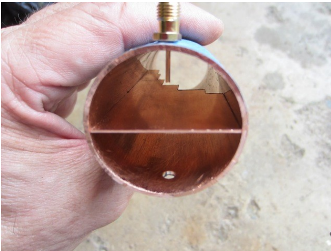
KNOWS 6 cm Feed Modified SM6FHZ Design
