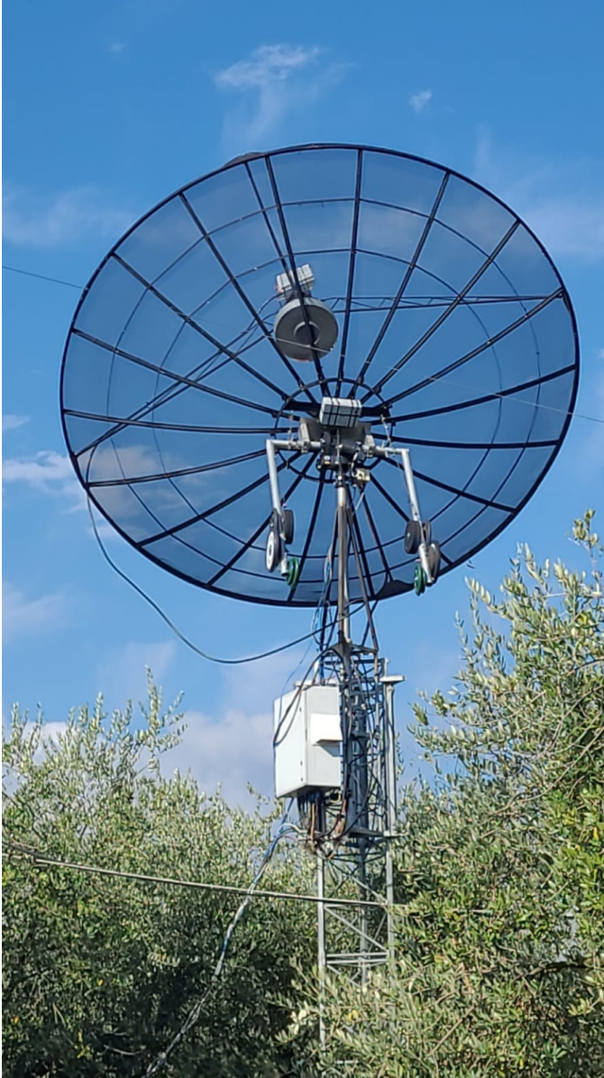
IK2DDR 3.7 m dish OM6AA feed ring
