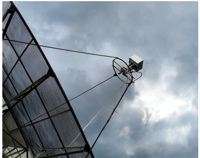
OH1LRY 3 cm system on 8 m dish
