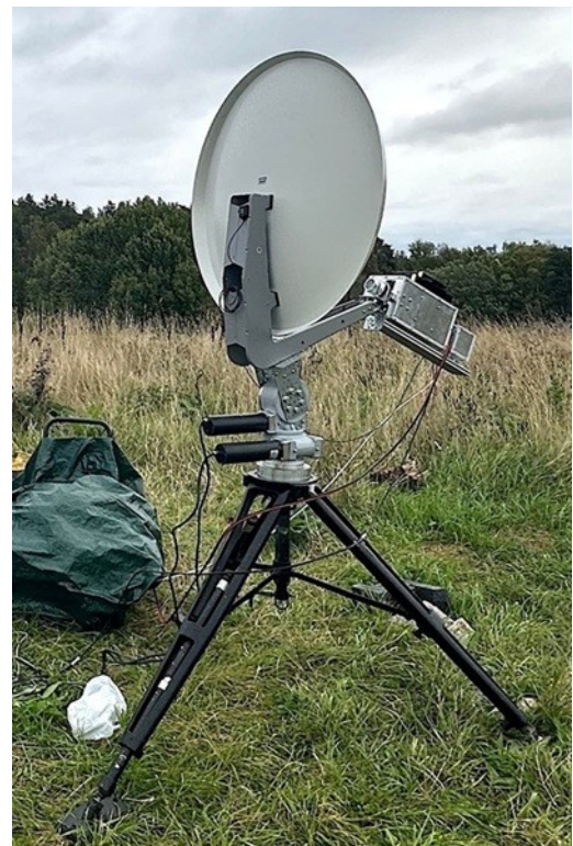
SA5IKN portable 10 GHz EME station
