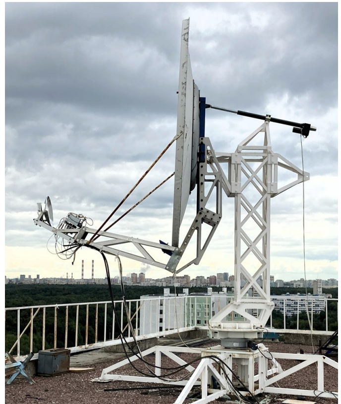
RW3BP 2.4 m antenna 76 GHz rig
