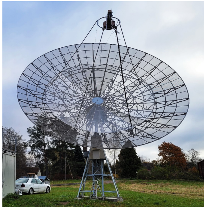
OH1LRY 23 cm system on 8 m dish
