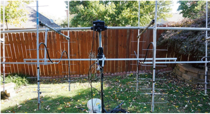
WD5AGO Closeup of Power Divider Harness
