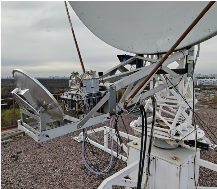
RW3BP 76 GHz Transverter at Feedpoint
