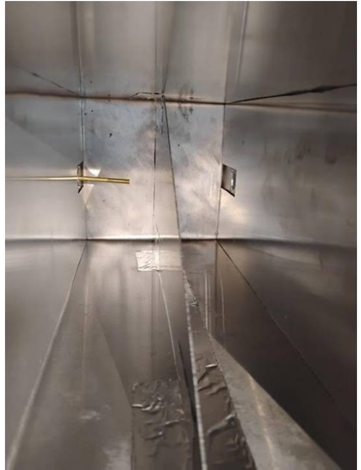
KNOWS - 3 - Feed Assembled with Aluminum Tape
