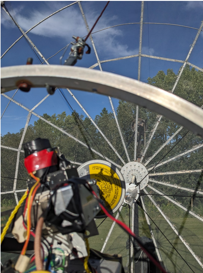
VE6TA 3 cm Feed with 20 degree offset
