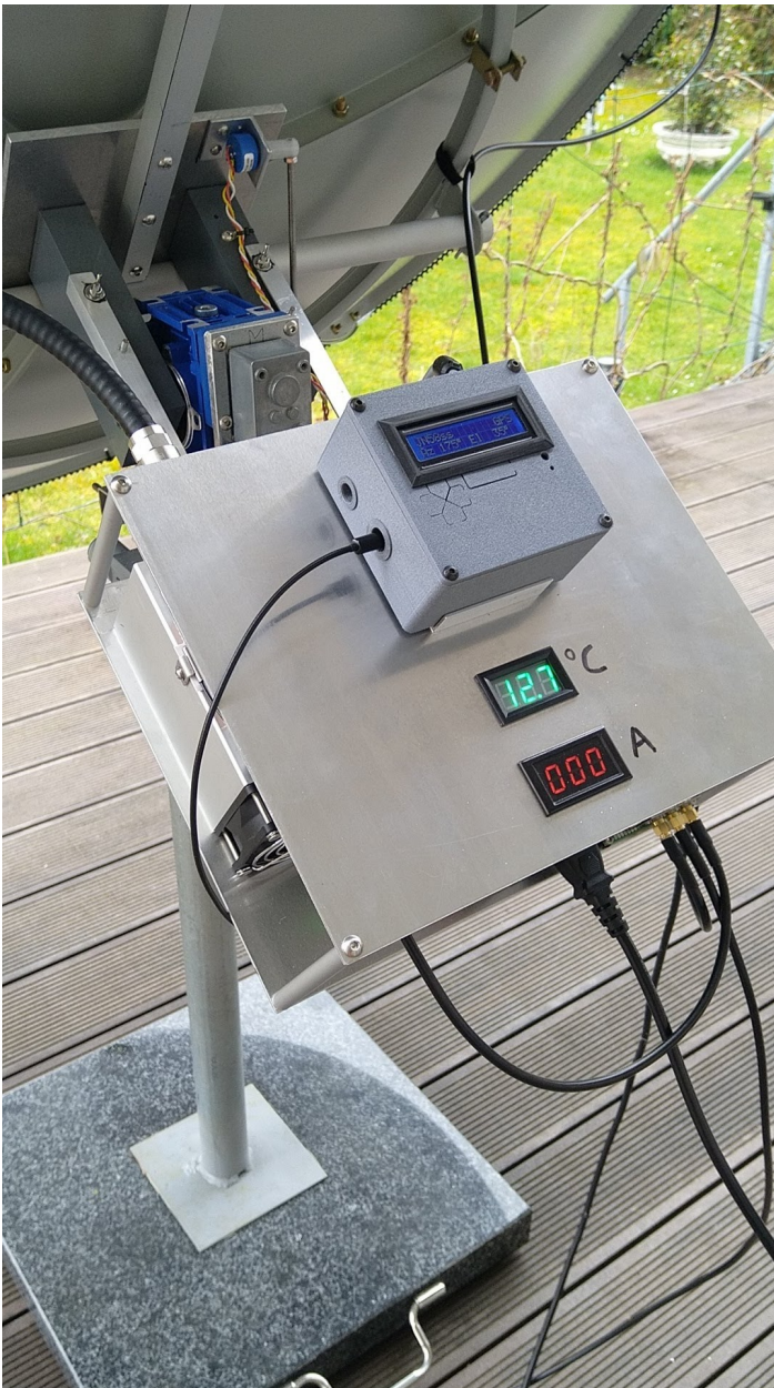
DC1RDP PA assembly antenna controller back of Cooker dish
