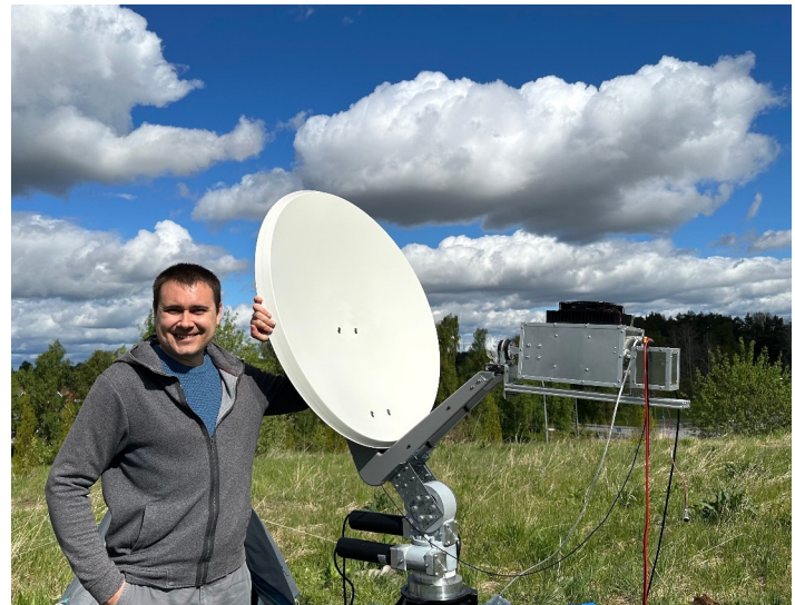
SASIKN portable OP with 90 cm dish 27 W on 2026-05-17
