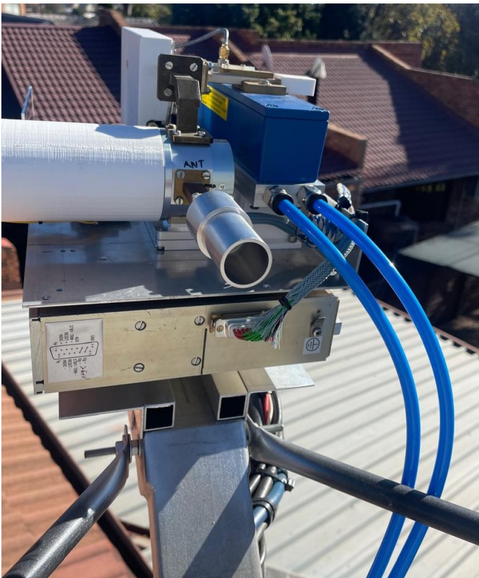
ZS6JON 24 GHz Water Cooling
