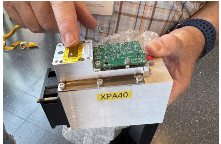
G4KLX Demo version of DU3T 40 W 3 cm PA at HAM RADIO
