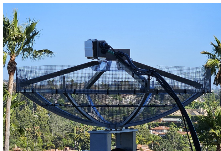
KB2SA 1 m Dish with Smaller Superpatch Feed
