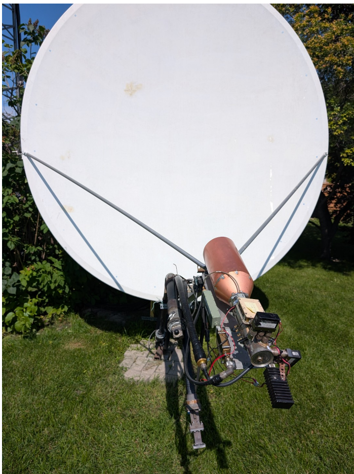
VE4MA 2.4 m Dish with 3.4 GHz Large W2IMU Feed
