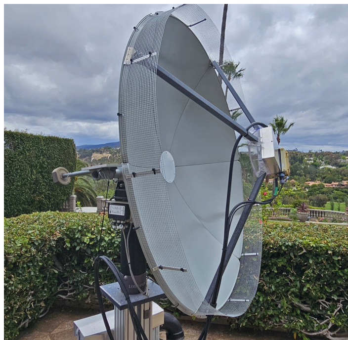
KB2SA Cooker Dish on 23 cm with Superpatch Feed
