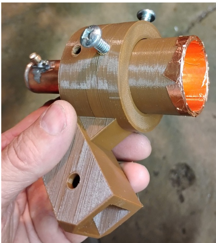
KNOWS 3D Printed W2IMU Feedhorn for 3 cm
