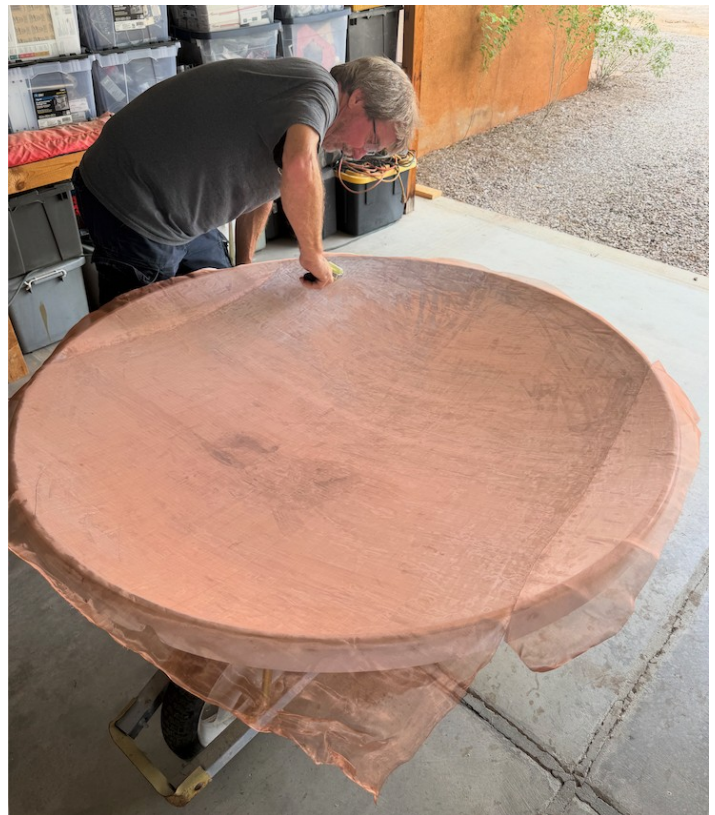
NJ6D Rolling Out the Copper Mesh on the 1.2 m Dish Surface
