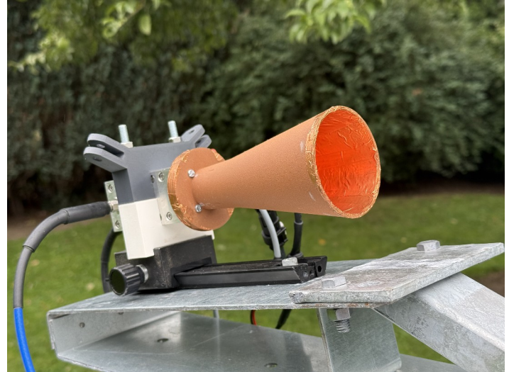
DL8EBL 3D Printed Skobolev 10 GHz Horn
