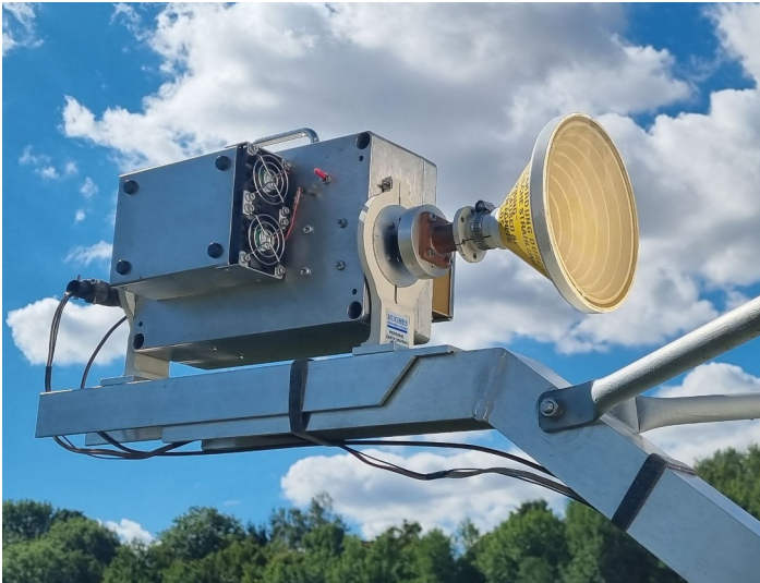
OK2AQ 3 cm Rotary Feed with 42 W SSPA 0.8 dB LNA and WG Switch
