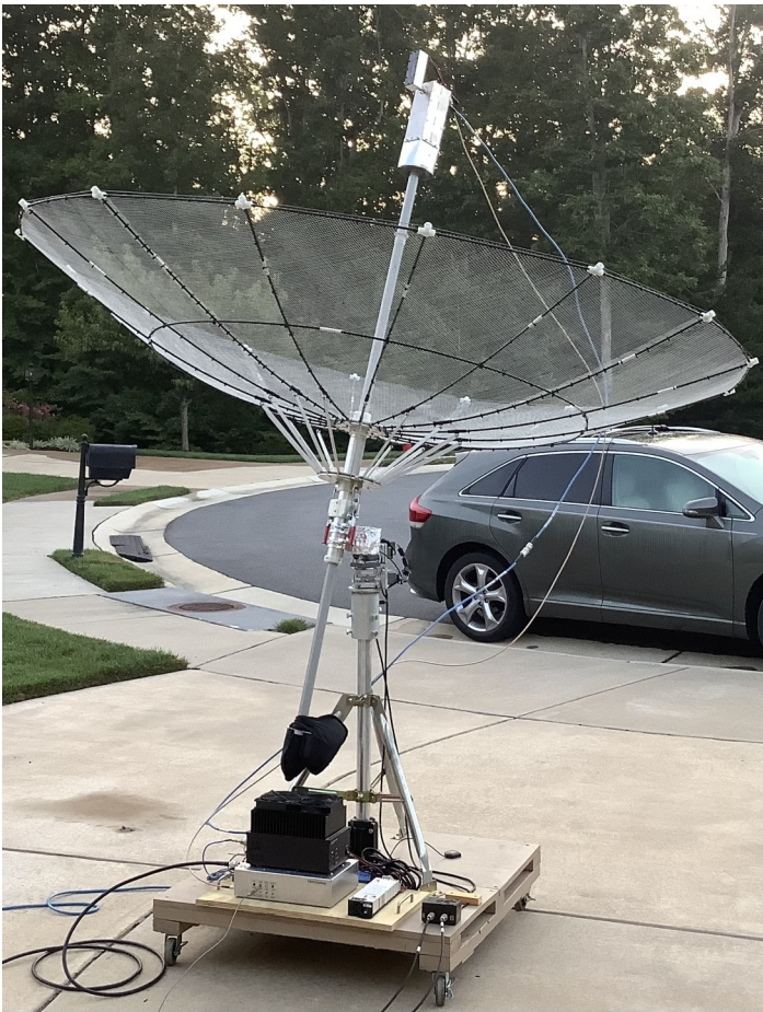
KN2K 2.3 m mesh dish 13 cm Septum Flare and S12 Disk
