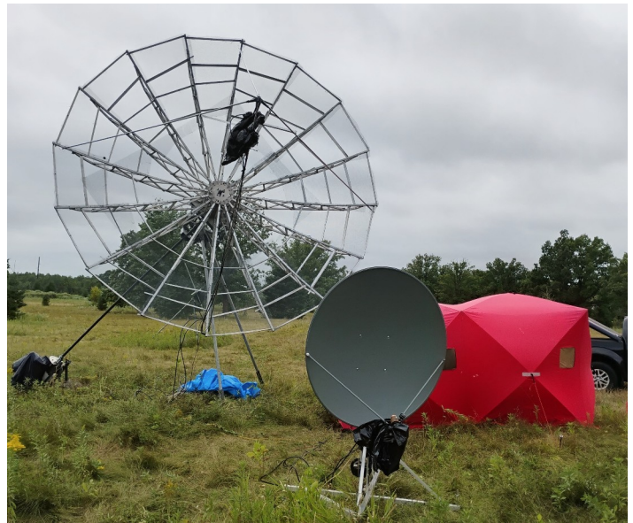
KNOWS Ready for 13 cm on the 4.8 m dish and 3 cm on the 1.2 m dish
