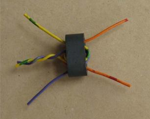
**L2, L3:** 40m Band-pass filter. 0.1 wire, 18 turns on the can former, spread in 3 slots.
