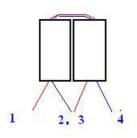
T1: Primary (yellow) 4 turns 0.38 wire or insulated wire on the binocular core; secondary (red) 2 turns, center tapped. See photo.
