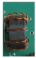
**T4:** IF transformer. Use 2 sleeves to form a binocular core. 0.31 wire, primary (crystal side) 5 turns, secondary 10 turns. It can be solder directly on the board,
