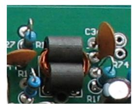
**T5:** Use the can former. 0.1 wire, primary (the 3-pin side) 16 turns, counter clockwise, the turns spread in 4 slots. Secondary (2-pin side), 4 turns in the bottom slot, counter clockwise. Wind the 2-pin side first. Pay attention to the start. See the illustration.
