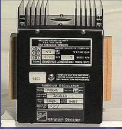
The FRK series were the best of the original types. All analogue, brute force physics package and well shielded. All discreet components. Mine still works fine. They are big in comparison to the LPRO. TTL or Sinewave output.
